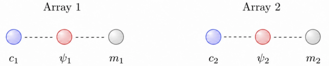
Figure 2: Two arrays, each containing a communication ion c , a target qubit state |\psi\rangle , and a memory ion m .
